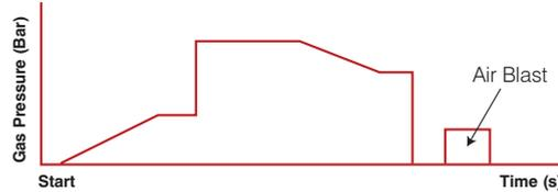
Advanced electromagnetic solenoid gas valves coupled with a sophisticated control system enable the operator to have effective control over the gas molding process. Up to five Pressure Profiles can be set with individual control of ramp and gas hold times available. An 'Air Blast' program may be included to ensure gas pins remain free from blockages.
